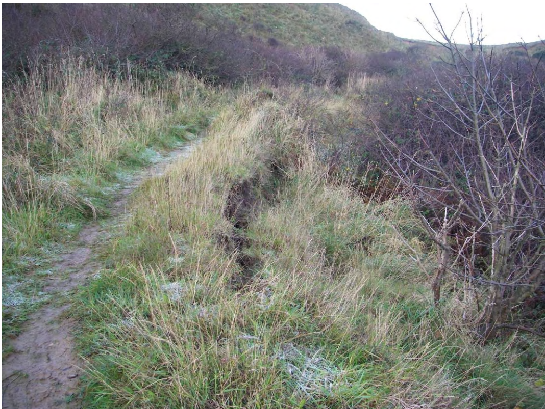
Plate 14. Site view of slopes showing mid-slope back rotated block and surface tension cracking.
